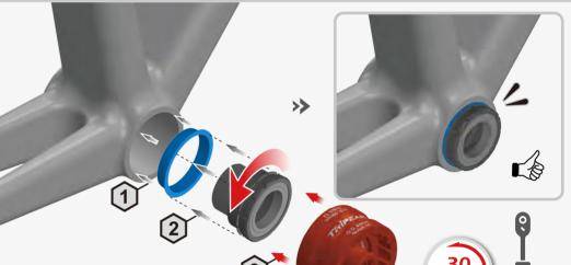
Remove the drive-side BB, which will be installed later.
